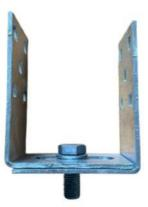
Adjustable L-brackets offer increased flexibility for using popular timber sizes in your foundation frame. Simply adjust the brackets to the required width, mount them on top of any M-profile ground screw, and secure with a bolt. These brackets also enable rotation, allowing you to align the timber in the desired direction.
